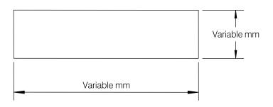
When thickness has to be reduced, the maximum width of this profile is 100mm.
