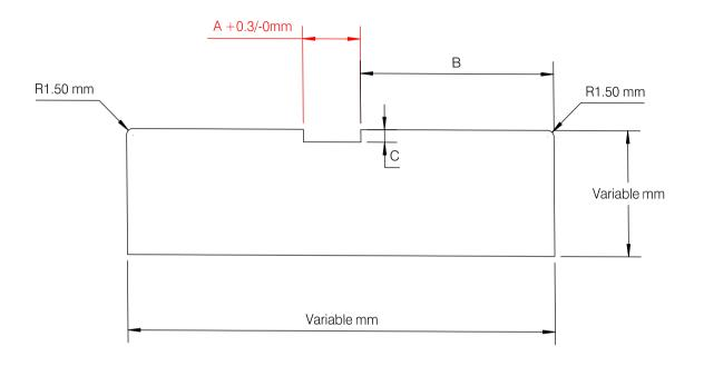
PLEASE NOTE: DIMENSION 'A' IS FOR INTUMESCENT STRIPS. PLEASE CHECK TO SEE IF THE GO/NO GO GAUGE FITS INTO GROOVE. 10mm, 15mm AND 20mm GO/NO GO GAUGES ARE AVAILABLE IN THE TOOLROOM.
